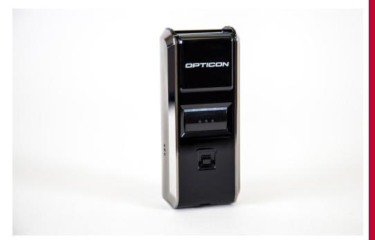
It is extremely compact and lightweight, making it ideal for mobile applications with a USB rechargeable lithium-ion battery. It can read 2D barcode formats and reads 1D barcode formats code 39, code 93 and code 128.
