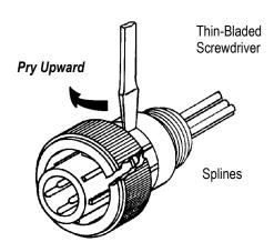
Removing Damaged Coupling Ring
