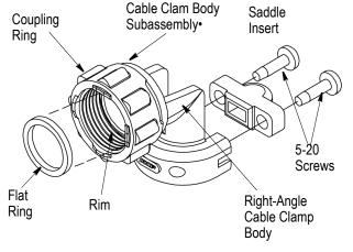
• The cable clamp body subassembly consists of the coupling ring ad the right-angle cable clamp body.
