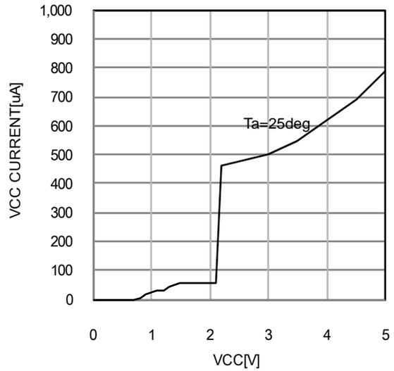
Fig.15 VCC input current vs VCC (STB ON)
