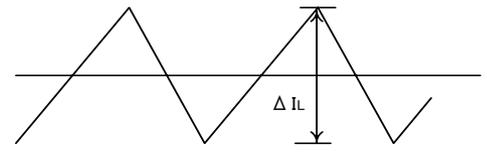
$$I_{peak} = \frac{V_{in} - V_{out} + V_f}{V_{in}} \times I_{out} + \frac{1}{2} \times \frac{V_{in} \times (-V_{out} + V_f)}{L \times f \times (V_{in} - V_{out} + V_f)}$$
