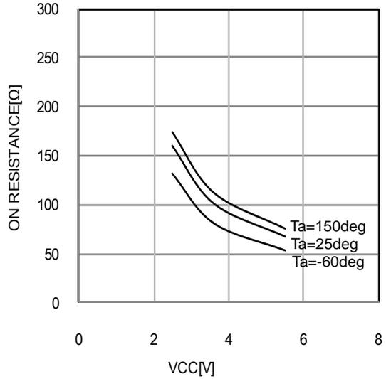
Fig.13 DIS1 discharge SW ON resistance vs VCC
