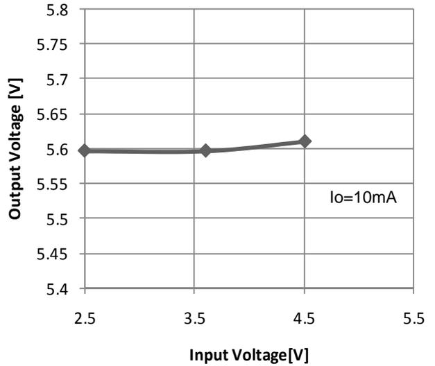
Fig.26 CH2 Output voltage vs Input voltage
