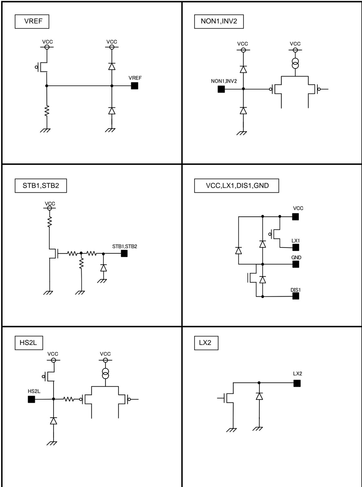
Fig.35 I/O Equivalence Circuit
