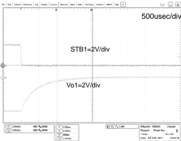
Fig.31 CH1 Discharge waveform [500usec/div]
