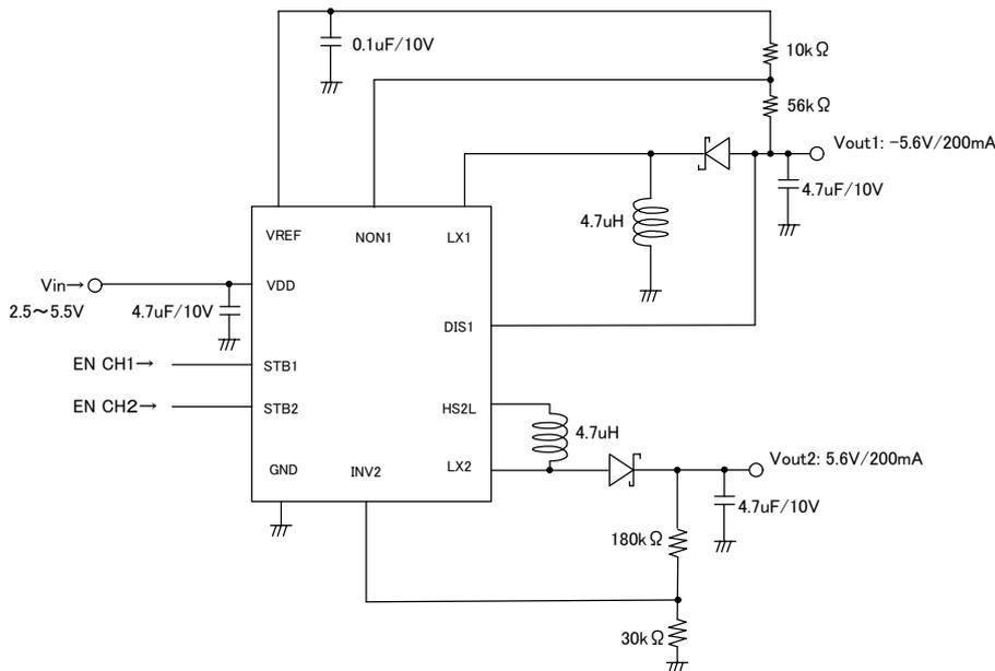
Fig.1 Application schematic
