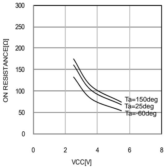
Fig.14 NON1 discharge SW ON resistance vs VCC
