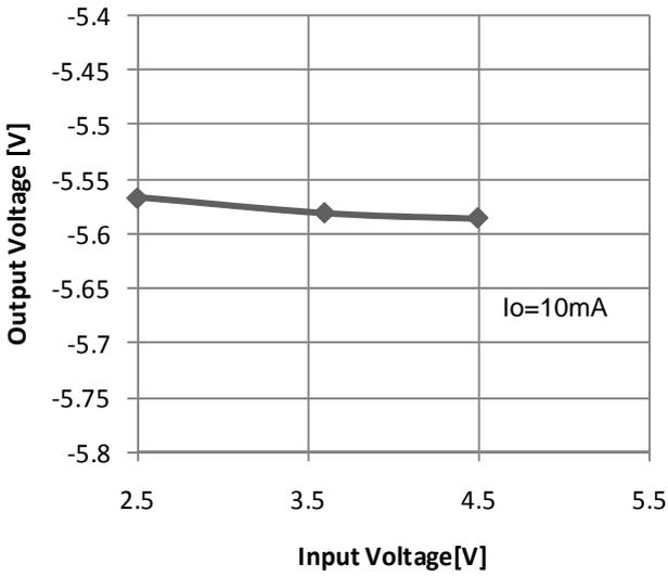
Fig.25 CH1 Output voltage vs Input voltage
