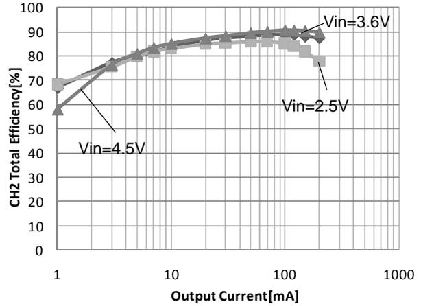
Fig.22 CH2 Power conversion efficiency vs output current
