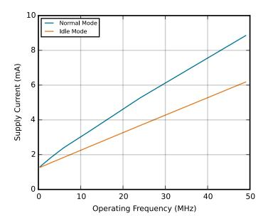
Figure 4.2. Typical Operating Supply Current using HFOSC1
