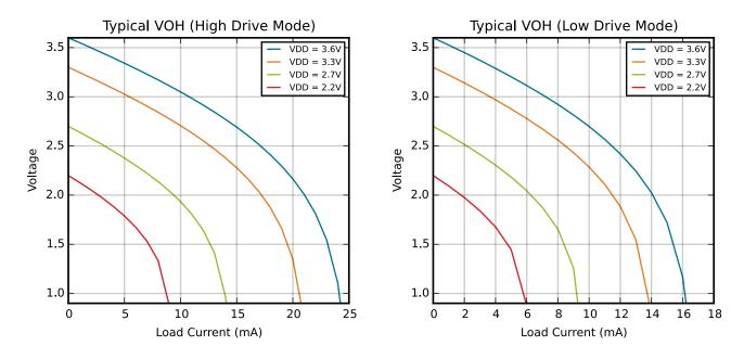
Figure 4.6. Typical V<sub>OH</sub> Curves
