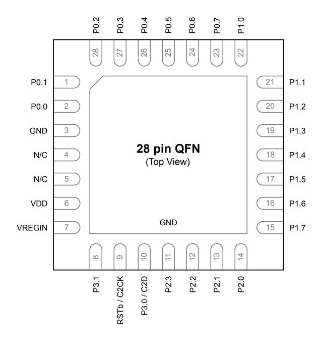
Figure 6.1. EFM8BB2x-QFN28 Pinout
