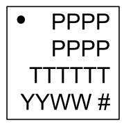
Figure 9.3. QFN20 Package Marking
