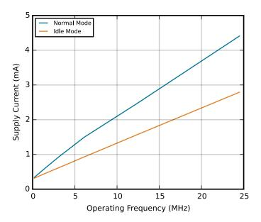
Figure 4.1. Typical Operating Supply Current using HFOSC0
