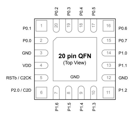
Figure 6.3. EFM8BB2x-QFN20 Pinout
