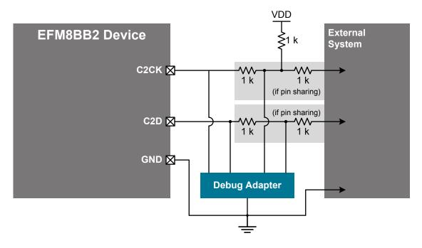
Figure 5.3. Debug Connection Diagram
