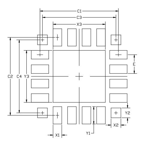
Figure 9.2. QFN20 PCB Land Pattern Drawing
