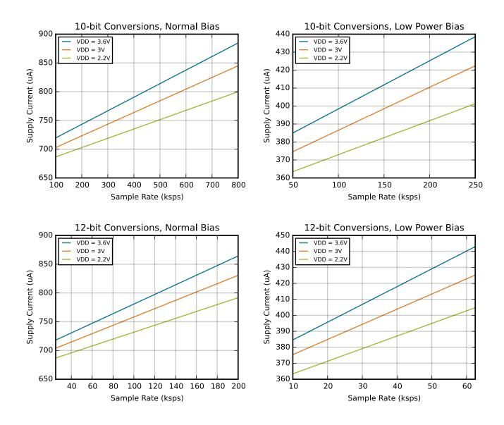
Figure 4.5. Typical ADC0 Supply Current in Normal (always-on) Mode
