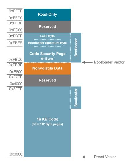
Figure 3.2. Flash Memory Map with Bootloader—16 KB Devices
