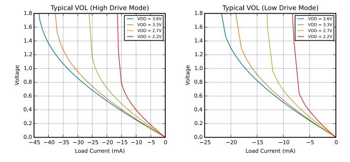
Figure 4.7. Typical V<sub>OL</sub> Curves
