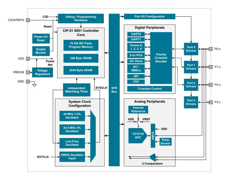
Figure 3.1. Detailed EFM8BB2 Block Diagram
