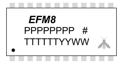
Figure 8.3. QSOP24 Package Marking
