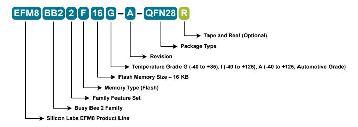
Figure 2.1. EFM8BB2 Part Numbering
