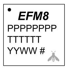
Figure 7.3. QFN28 Package Marking
