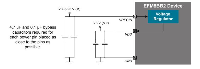
Figure 5.1. Connection Diagram with Voltage Regulator Used
