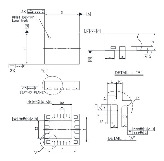
Figure 9.1. QFN20 Package Drawing
