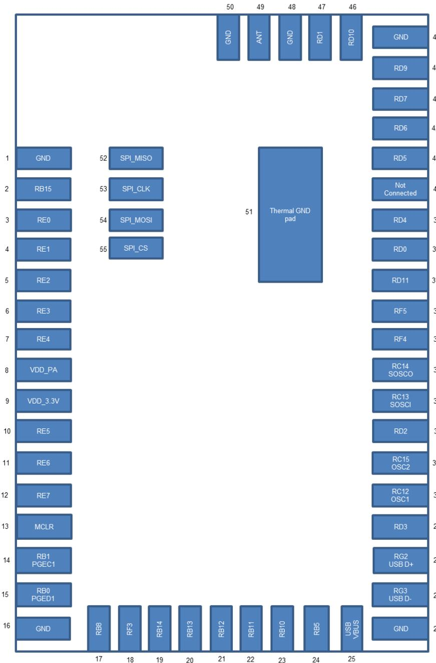
Figure 1: WF121 pinout
