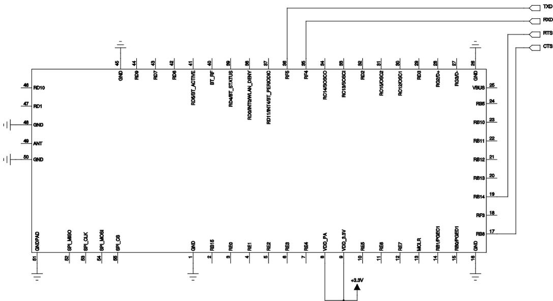
Figure 6: Minimal system required for UART host connection
