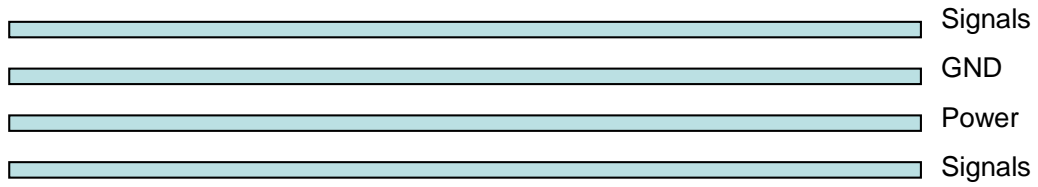
Figure 17: Typical 4-layer PCB construction
