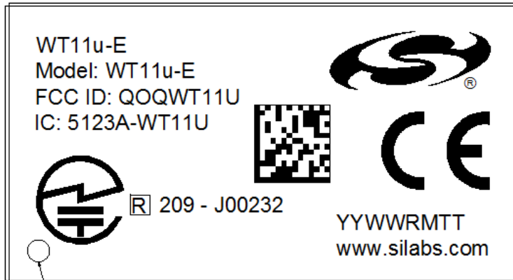
Figure 33: WT11u-E package marking
