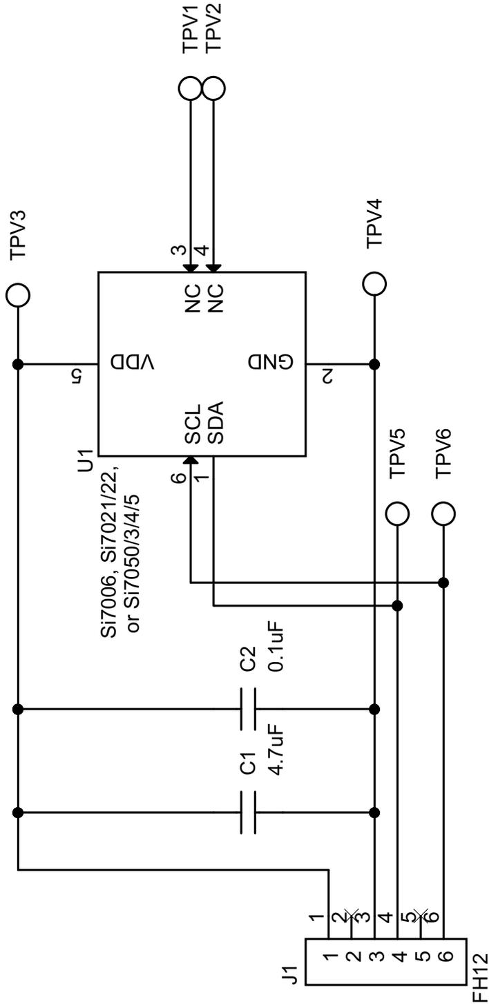
Figure 16. Si7006, Si7020/21, or Si7050/3/4/5 EB Schematic
