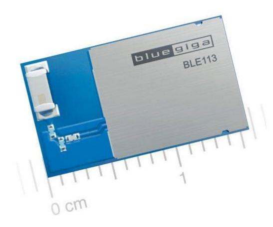
The BLE113 is a Bluetooth Smart module targeted for small and low-power sensors and accessories. It integrates all features required for a Bluetooth Smart application, including Bluetooth radio, software stack, and GATT-based profiles. The BLE113 Bluetooth Smart module can also host end-user applications, which means no external microcontroller is required in size or price constrained devices. Moreover, it has flexible hardware interfaces to connect to different
