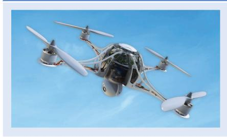
Vibrations and shocks cause blurring on optical systems such as cameras. This blurring effect can be reduced by mechanical stabilization: A gyro is used to measure the movement and a microcontroller directs that signal to small linear motors compensating for the motion. The control loop should run sufficiently fast in order to resolve the vibrations and provide enhanced image capabilities. Tronics sensors provide an adequate data rate and reduced latency down to 1 ms.
