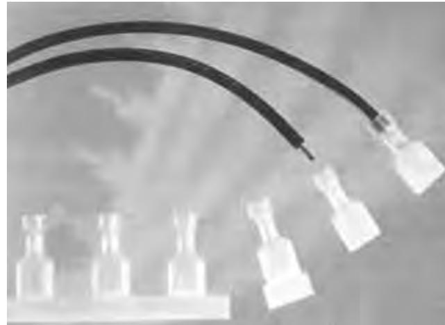
housing are molded from type 6/6 nylon material with a +130°C UL temperature rating. The insulation barrel is molded from a premium grade nylon selected to retain the insulation crimp shape. This premium nylon exhibits minimal springback, thus providing actual insulation crimp tensile strength as well as strain relief for applications where extreme wire dressing and/or vibration are present.
