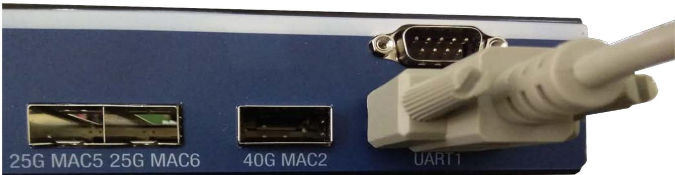
**Figure 8. Console connection**
