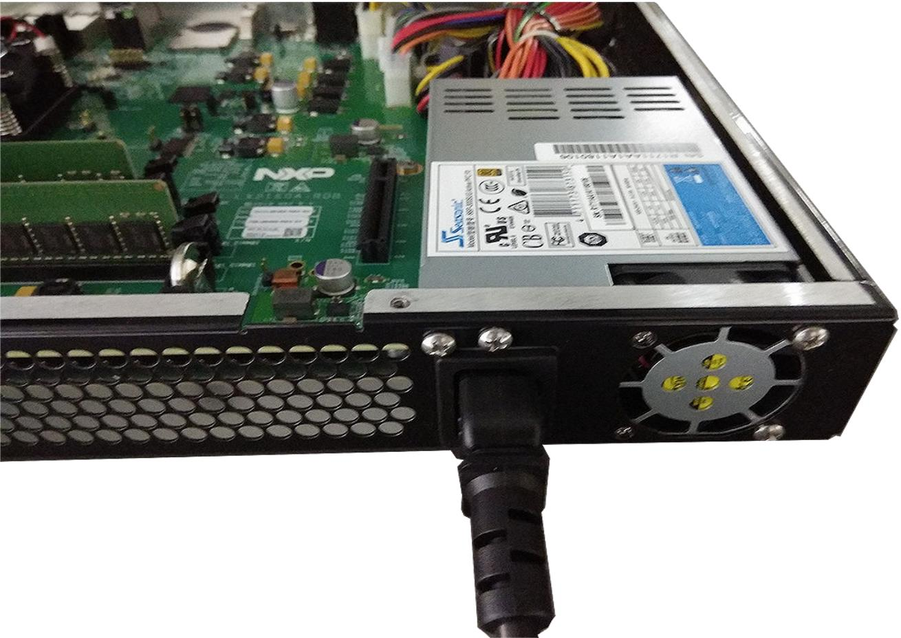
**Figure 6. Power supply connection**
