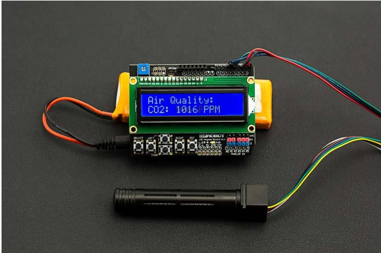
[DFRobot LCD Keypad Shield](#) with UART Infrared CO2 Sensor
