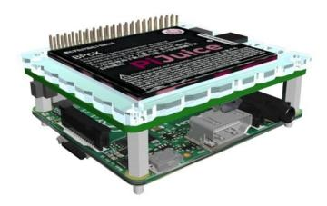
The PiJuice is an uninterrupted power supply board for Raspberry Pi. It has onboard 1400mAh off the shelf Li-Po / Li-ion battery for approximately 6hours in constant use (with support for larger Li-Po Battery of 5000mAH or 10,000mAH + to last up to 24hrs).
