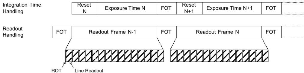
Figure 12. Integration and Readout for Pipelined Shutter
