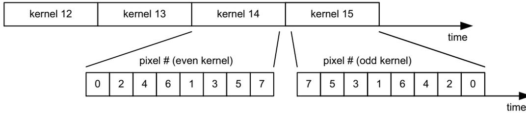
**Figure 47. P2–SN/SE: Data Output Order without Subsampling**
