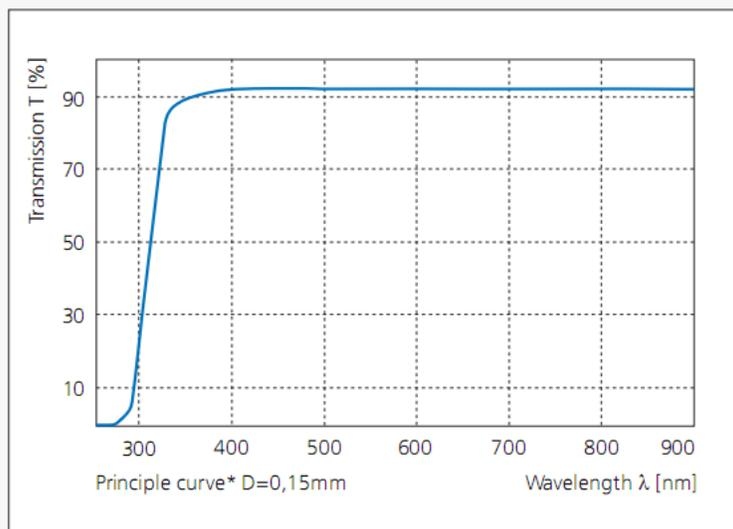
Figure 55. Transmission Characteristics of the Glass Lid
