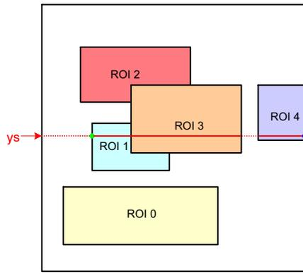
Figure 28. Scanning the Image Array with Five Windows
