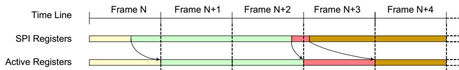
**Figure 20. Frame Synchronization of Configurations (no freezing)**
