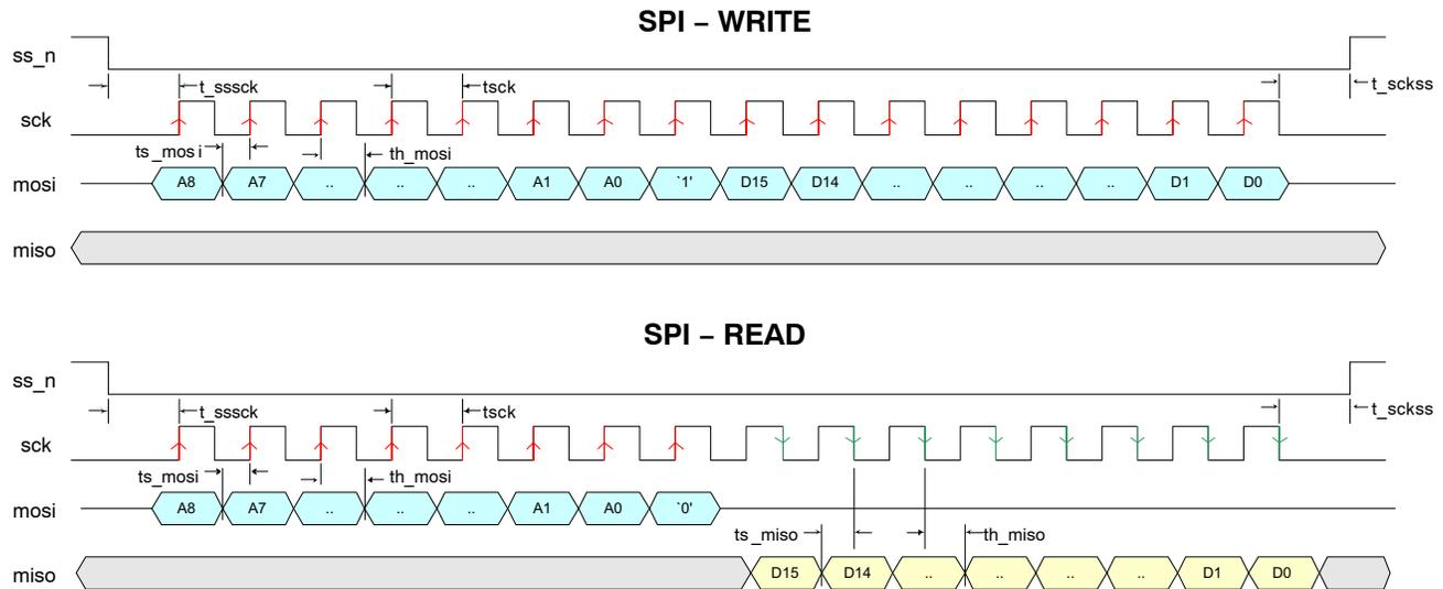
**Figure 22. SPI Read and Write Timing Diagram**
