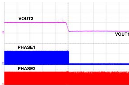
Figure 6. VOUT2 Tracking VOUT1 when Channel 1 is Disabled
