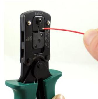
Insert the cable until insulation Stop blade.
