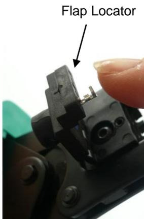
Contact has to be inserted to the stop.
