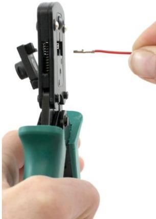
Remove the crimped contact.
