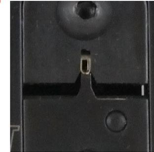
Close the tool lightly until the contact is held (1. Ratchet Lever)
