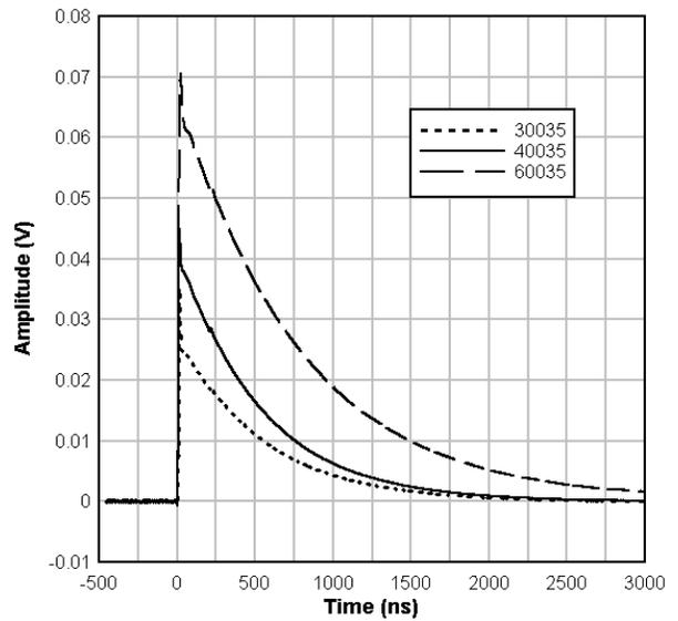
**Figure 6. Standard Output Pulse Shape**
