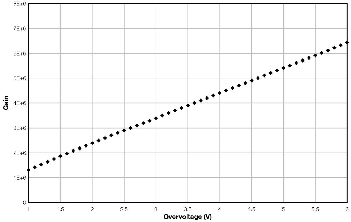
**Figure 4. Gain vs. Overvoltage**
