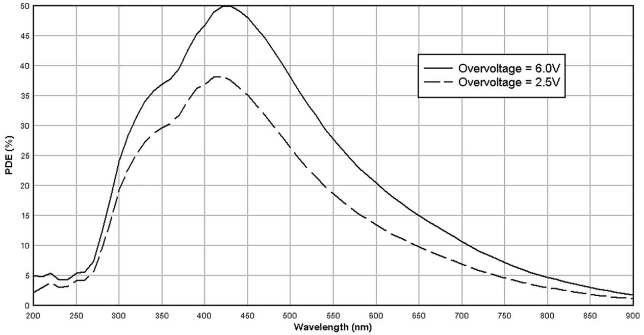
**Figure 1. Photon Detection Efficiency (PDE)**
