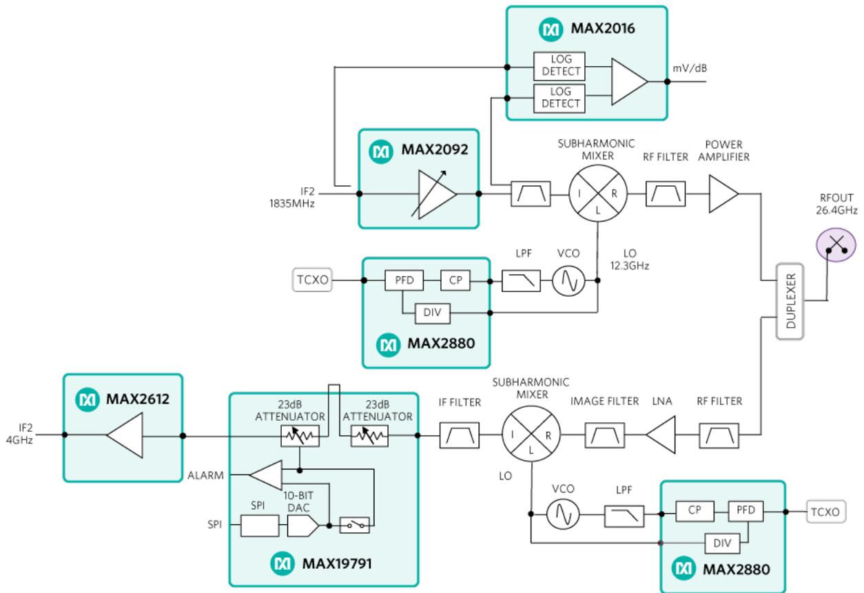
Figure 3. Schematic for the microwave up/down frequency converter section in a split mount ODU.
