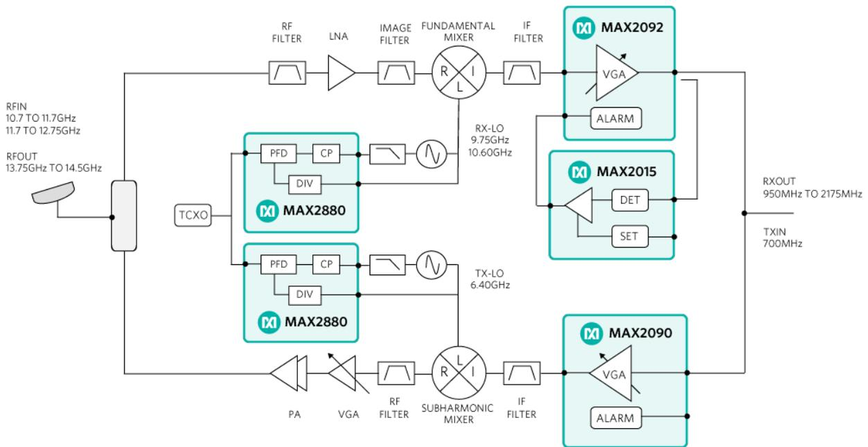
Figure 11. Analog RF building blocks play an important role in VSAT ODU microwave radios. Here the LNB and BUC rely on PLL frequency synthesizers and high-linearity VGAs for stable performance over temperature extremes.
