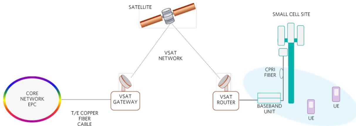
*Figure 10. Satellite backhaul with a broadband VSAT system connects a remote small cell base station to the core network.*
