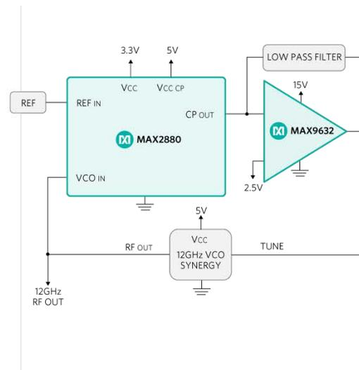
*Figure 8. Phase noise is an important PLL-frequency-synthesizer performance metric in LO applications. For simplicity, passive R-C components for filtering, AC-coupling, and impedance matching are excluded at the lowpass filter for the MAX2880.*
