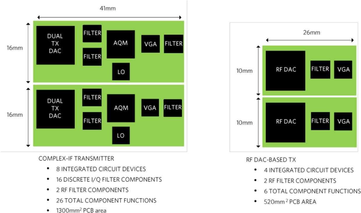
Figure 7. PCB area comparison of a complex-IF versus RF DAC transmitter supporting CCDP or 2x2 MIMO. The RF DAC transmitter (right) significantly reduces PCB area and component count. AQM = analog quadrature modulator; LO = local oscillator (PLL/VCO synthesizer); VGA = variable gain amplifier; I/Q filters = multipole, differential. Diagram not to scale.
