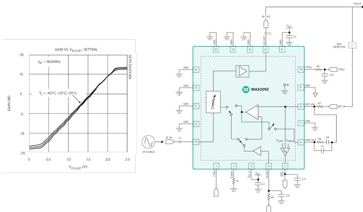
Figure 9. An important VGA feature is high linearity over a wide operating temperature range with precise linear-in-dB level control (shown in the performance curves on the left). A VGA, like the MAX2092, is a common RF building block used for ATPC applications and RX-TX signal leveling.
