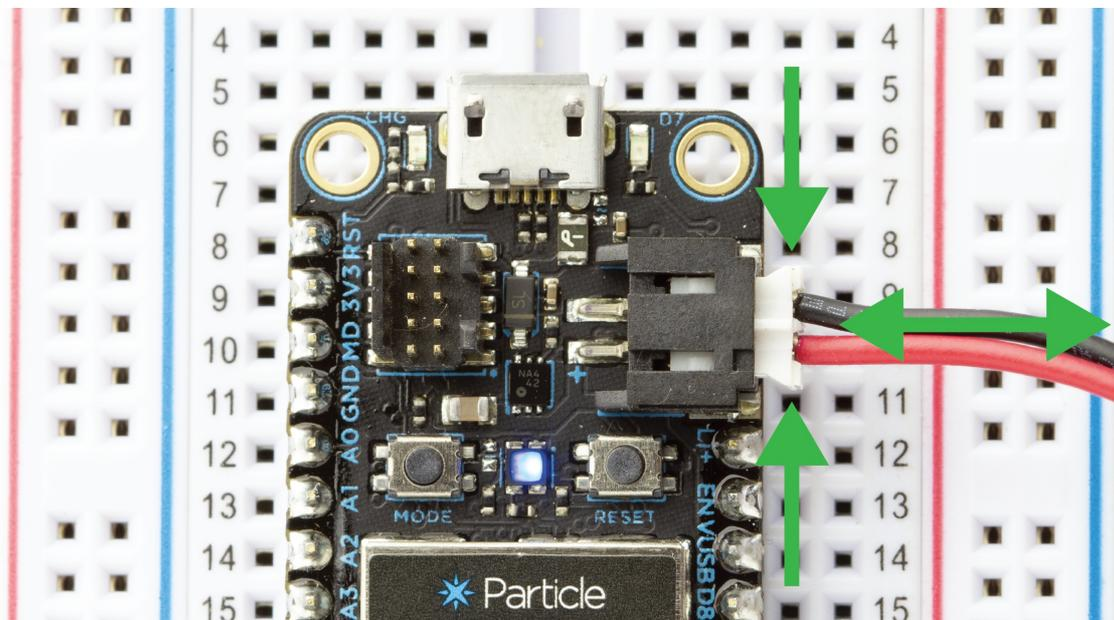
The micro B USB connector on the Argon is soldered on the PCB with large surface pads as well as couple of through hole anchor points. Despite this reinforcement, it is very easy to rip out the connector if too much stress is put on in the vertical direction.
