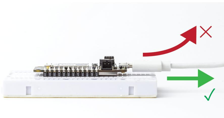
The u.FL antenna connector is a very fragile piece of hardware ( and is fancy too with all the gold plating). The connector was not designed to be constantly plugged and unplugged. Care must be
