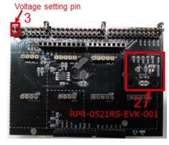
Figure 2. Connection between RPR-0521RS-EVK-001 and the SensorShield
