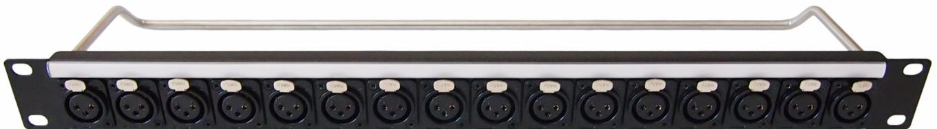
**CP30182** - 1U Panel loaded with 16 x XLR 3DCF . M3 Holes. Front mounted
