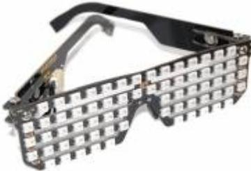
RGB Shades are a wearable LED matrix shaped like slotted sunglasses. The current version was developed as the result of a [Kickstarter campaign](https://www.kickstarter.com/projects/macetech/rgb-led-shades) [https://www.kickstarter.com/projects/macetech/rgb-led-shades] and are currently available for sale on [macetech.com](http://macetech.com)
