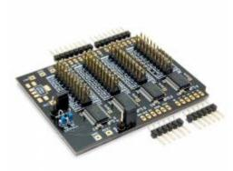
The Centipede Shield [http://macetech.com/store/index.php? main\_page=product\_info&cPath=4&products\_id=23] is an add-on PCB for standard layout (Uno, Duemilanove, Diecimila) Arduino microcontroller boards. It uses the Wire I2C interface on analog pins 4 and 5 to provide 64 general purpose I/O pins. Any pin can be configured for input or output. The shield uses four Microchip MCP23017 [http://www.microchip.com/wwwproducts/Devices.aspx? dDocName=en023499] 16-pin digital I/O expander chips.
