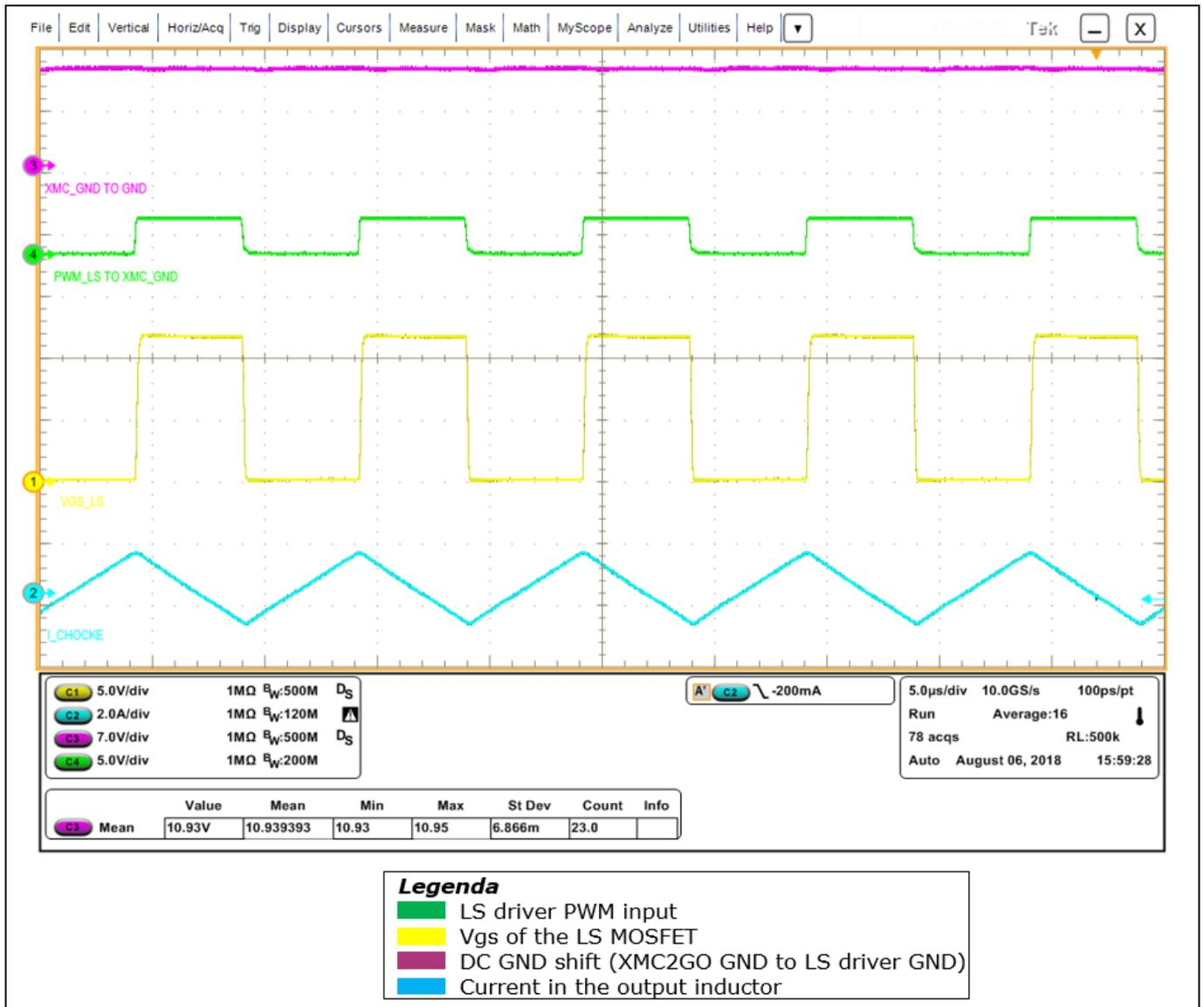
**Figure 8** Waveforms confirming the proper 1EDN8550B driving of the LS MOSFET with 10.93 V generated DC GND offset
