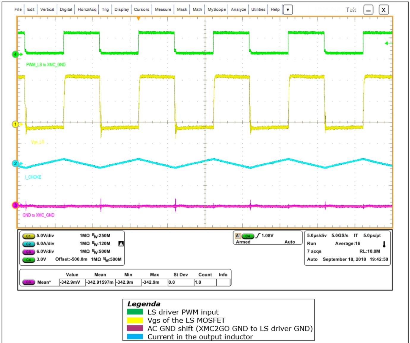
**Figure 16** Waveforms showing the board running using the standard single-channel 1EDN8511B as LS driver with 0 V DC GND shift between the microcontroller GND and the LS driver GND
