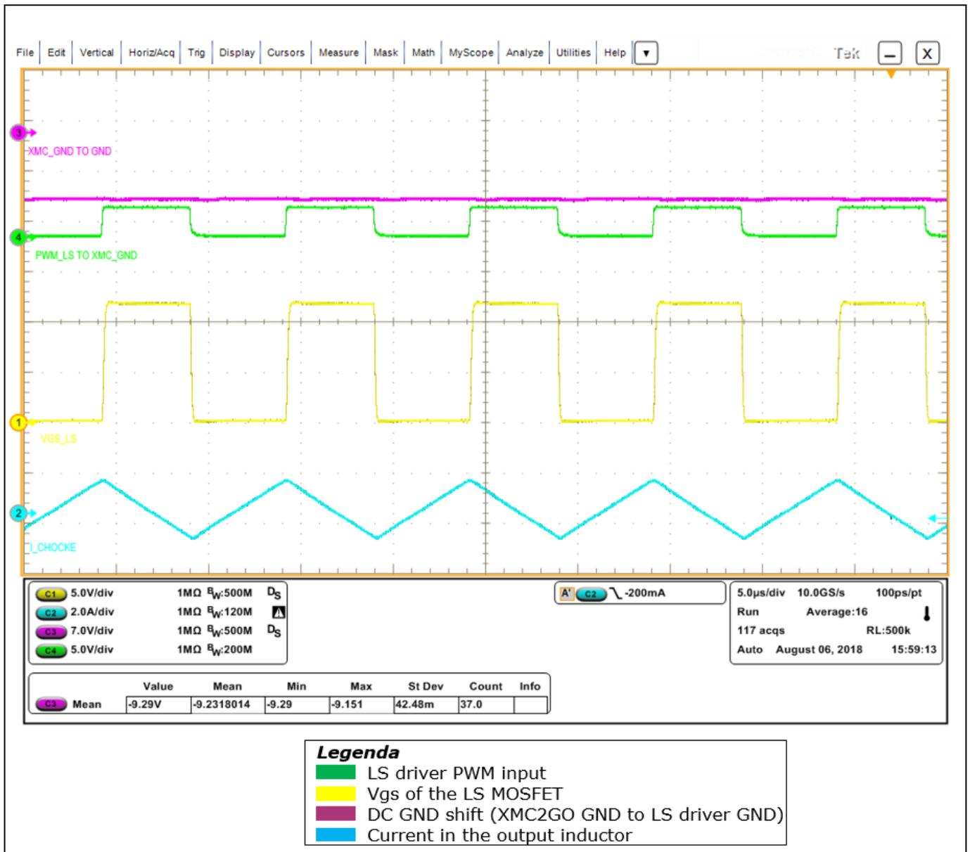
**Figure 6** Waveforms confirming the proper 1EDN8550B driving of the LS MOSFET with -9.3 V DC GND offset
