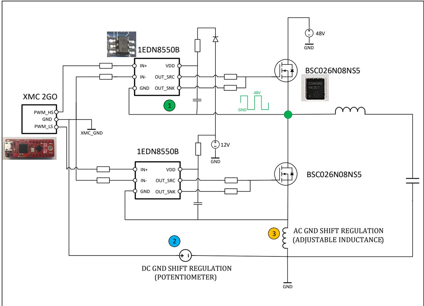
**Figure 2** TDI HB BC evaluation board – basic block diagram showing the Infineon products used and the major sections of interest
