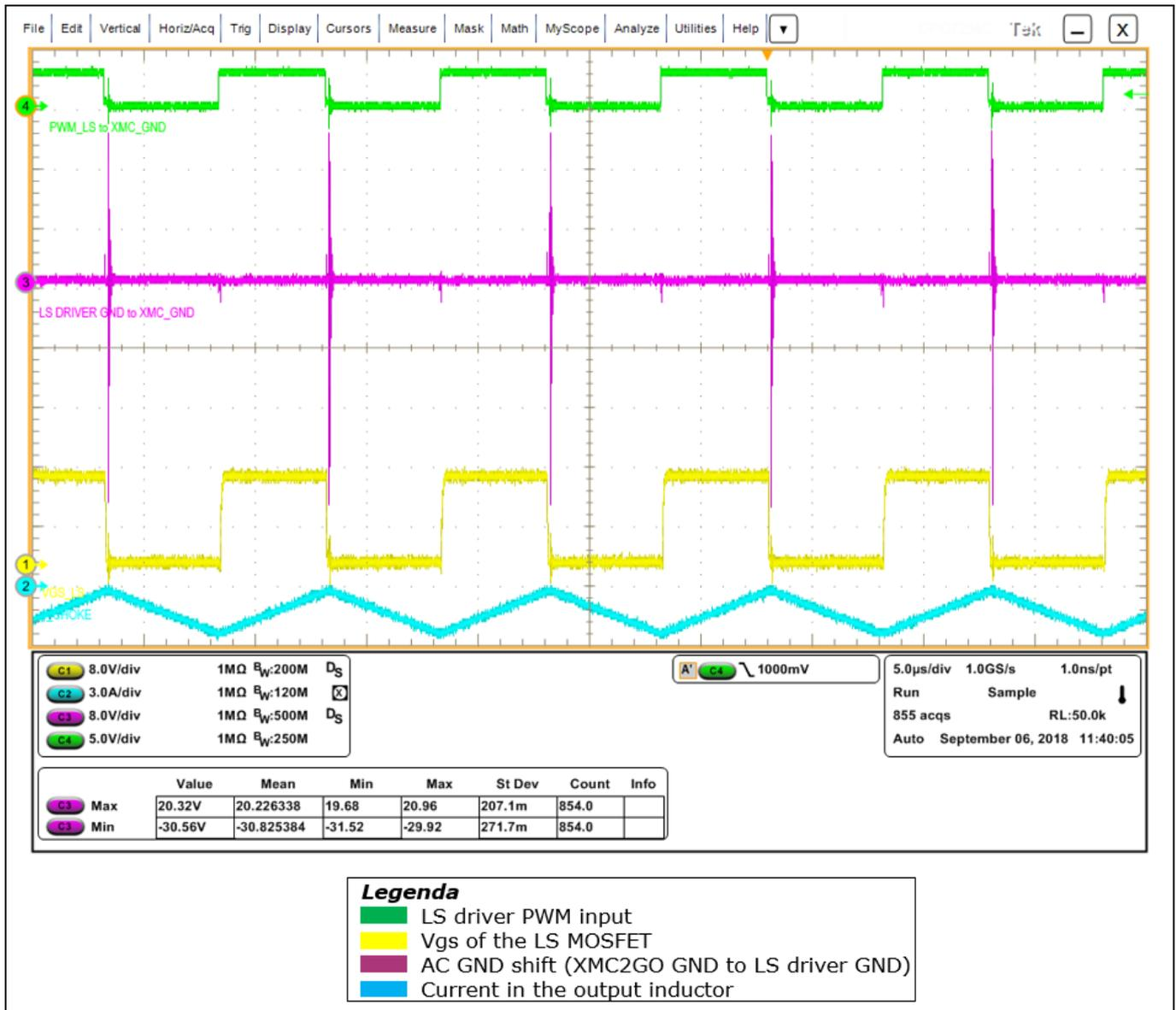
**Figure 10** HB BC evaluation board waveforms obtained using the 1EDN8550B as LS driver with 18  $\Omega$  load and in the worst configuration of GND inductance showing the TDI driver immunity to AC GND shifts
