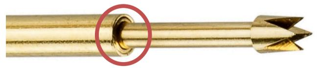
The resistance felt during the insertion is the probe body pressing past the indent in the sleeve – this will retain the probe in the sleeve once the probe is fully inserted.
