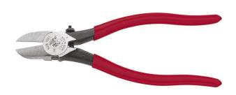
Precisely cuts injection mold sprues, gates and other plastic. Adjustable 1/16-Inch (2 mm) hollow-head screw keeps knife-edges from damaging each other. Spring-loaded for self-opening action. Flush cutting knives. Not designed for use on metal.
