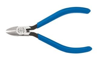
Tapered nose for easy working in confined areas and close tip cutting. Short jaws and beveled cutting edges permit close cutting of wire. Induction-hardened cutting knives for long life. Hot-riveted joint ensures smooth action and no handle wobble. Plastic-dipped handles for comfort and ease of identification. Custom, US-made tool steel.
