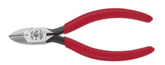
"W" notches to cleanly slit insulation. "V" notch at hinge for quick insulation crushing. Tapered nose for easy working in confined areas and close tip cutting.
