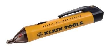
Use this Non-Contact Voltage Tester to detect standard voltage in cables, cords, circuit breakers, lighting fixtures, switches, electrical sockets and wires. A bright-green LED will tell you that the tester is working, and also functions as a work light. It changes to red, and warning tones sound, when voltage is detected.
