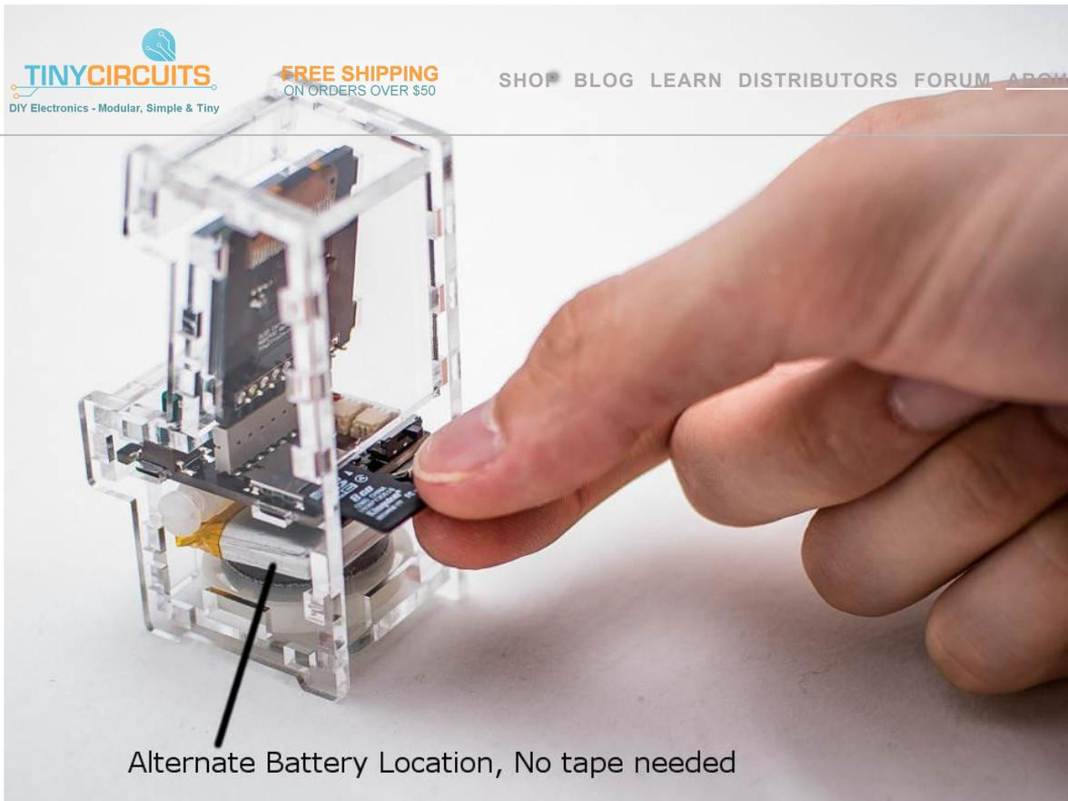
Alternate Battery Location, No tape needed
