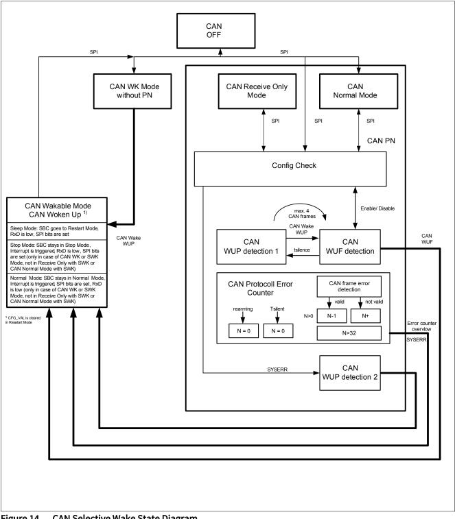
Figure 14 **CAN Selective Wake State Diagram**
