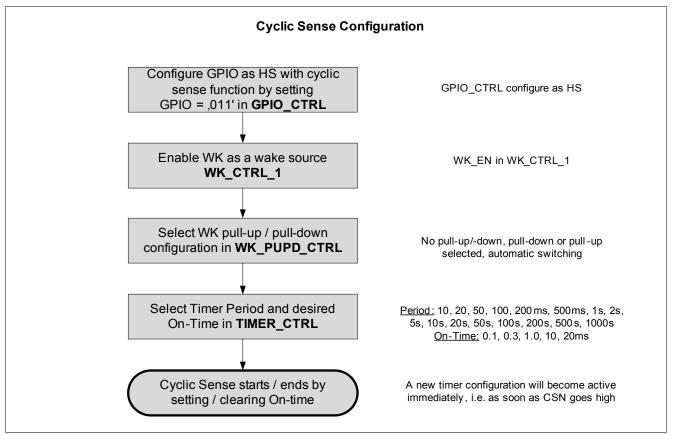
Figure 7 Cyclic Sense: Configuration and Sequence
