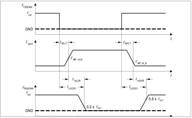
Figure 28 Timing Diagrams for Dynamic Characteristics
