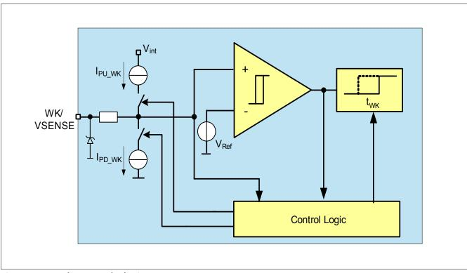
Figure 30 Wake Input Block Diagram
