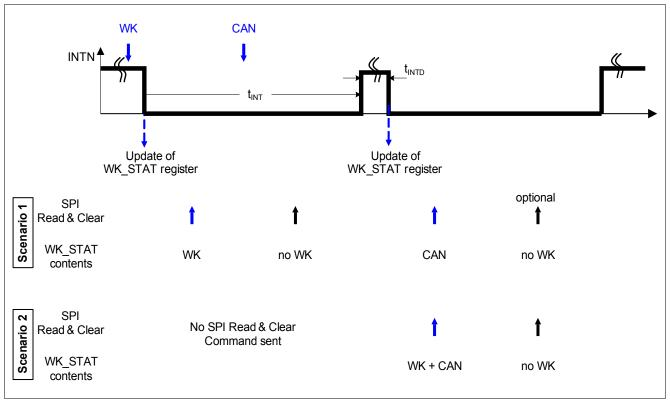
Figure 34 Interrupt Signalization Behavior
