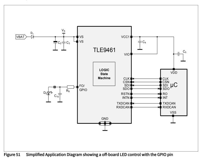
Note: This is a very simplified example of an application circuit. The off-board LED control function must be verified in the real application. The external circuitry is a minimum requirement and may vary depending on respective requirements. The same protection requirments apply for the configuration of FO/GPIO as low-side switch or wake input.
