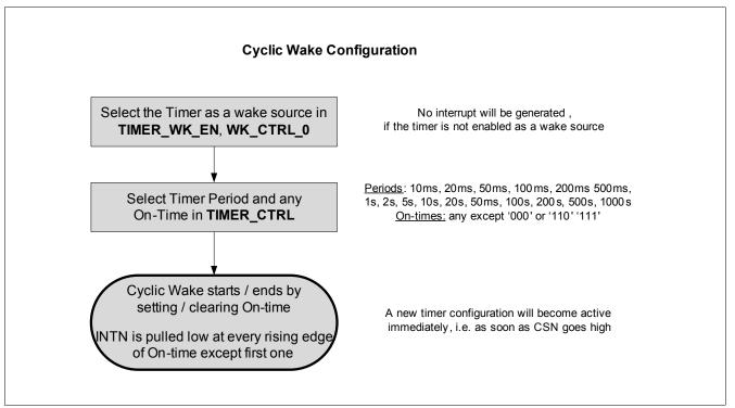
Figure 11 Cyclic Wake: Configuration and Sequence
