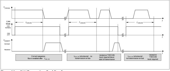
Figure 26 CAN Transceiver Enabling Sequence
