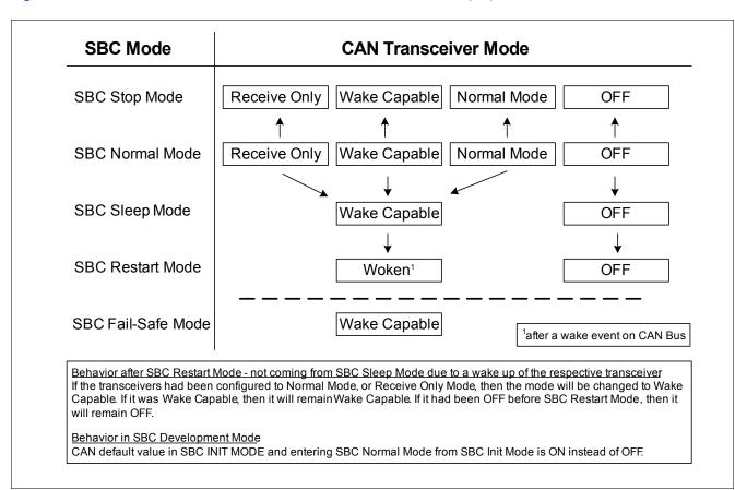
Figure 24 shows the possible transceiver mode transition when changing the SBC mode.
