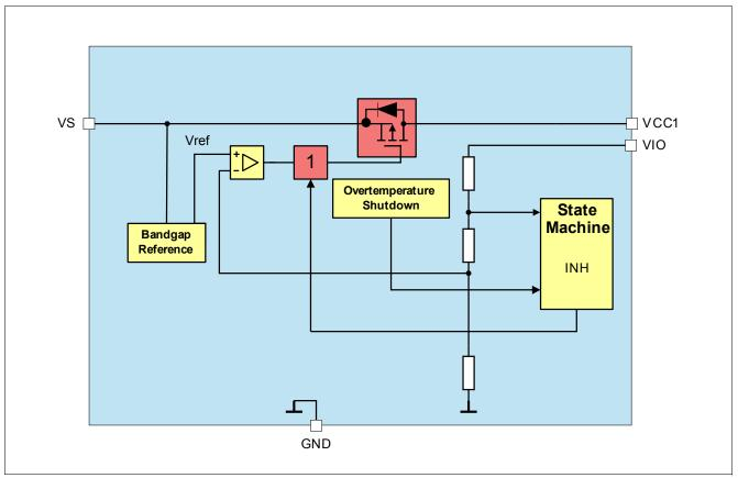
Figure 19 Module Block Diagram
