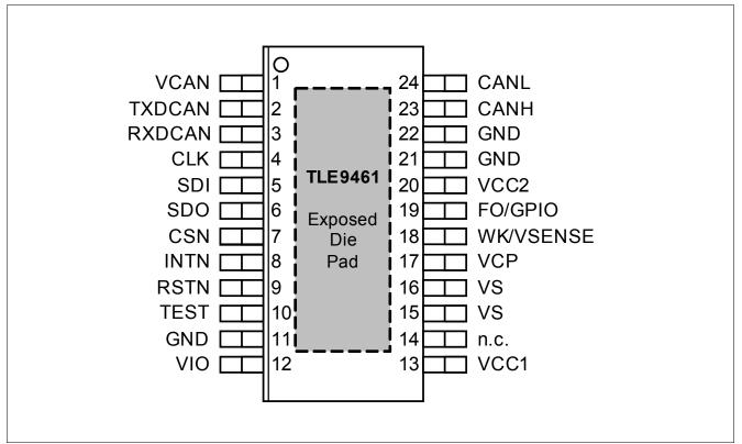
Figure 2 Pin Configuration
