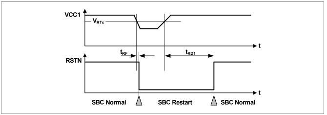
Figure 42 VCC1 Undervoltage Timing Diagram
