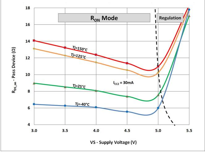
Figure 21 Typical on-resistance of VCC2 pass device during linear (R<sub>ON</sub>) mode for /<sub>CC2</sub> = 30mA
