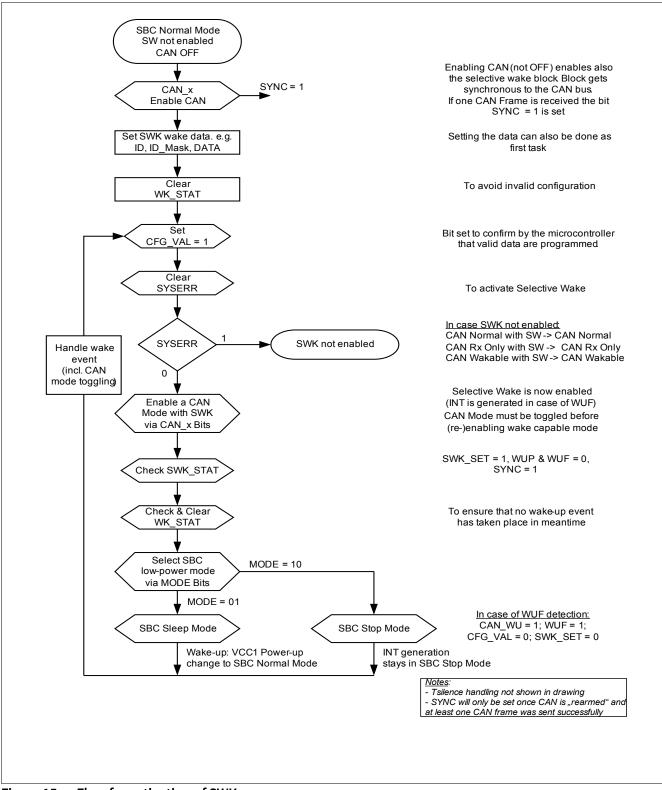
Figure 15 Flow for activation of SWK
