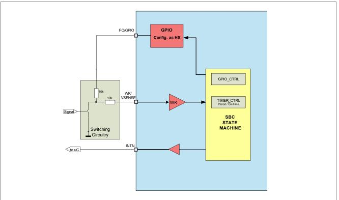
Figure 6 Cyclic Sense Working Principle
