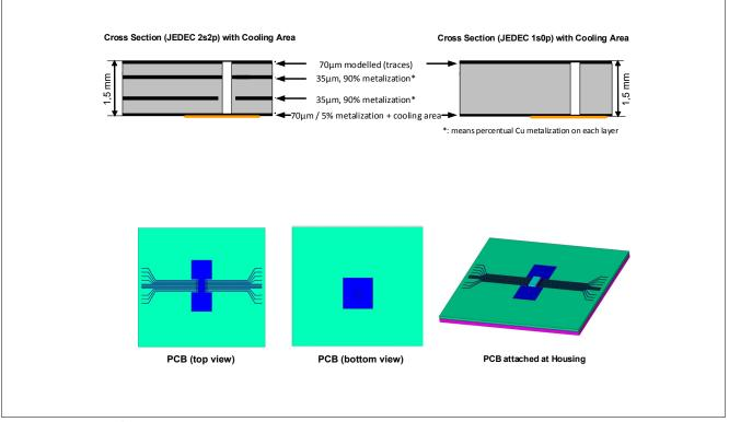
Figure 55 Board Setup
