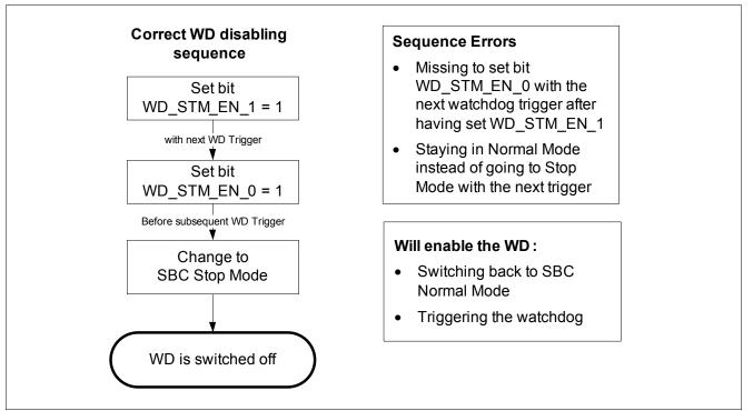
Figure 40 Watchdog disabling sequence in SBC Stop Mode
