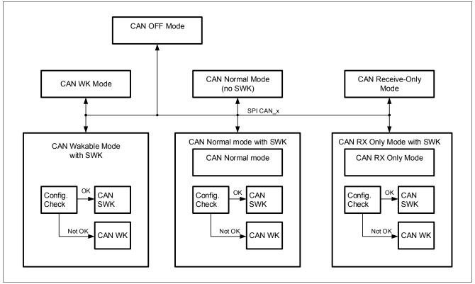
Figure 17 CAN SWK State Diagram
