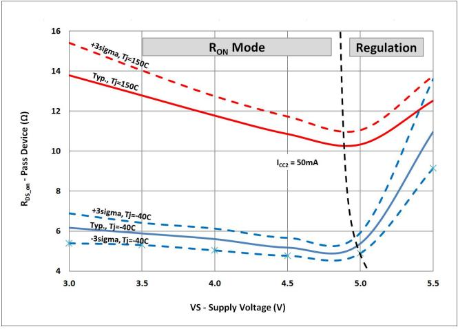
Figure 22 On-resistance range of VCC2 pass device during linear ( $R_{ON}$ ) mode for  $/_{CC2}$  = 50mA
