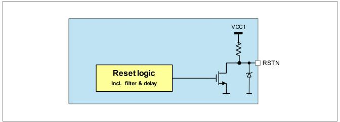
Figure 36 Reset Block Diagram
