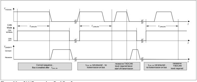
Figure 26 CAN Transceiver Enabling Sequence
