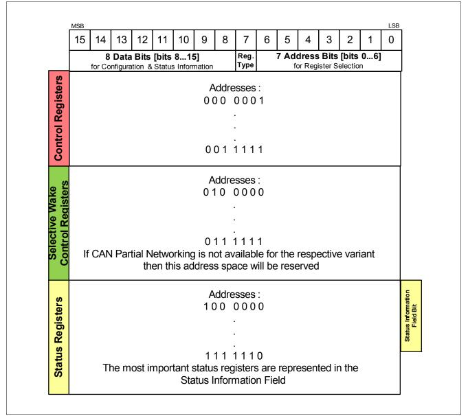
Figure 47SPI Register Mapping Structure
