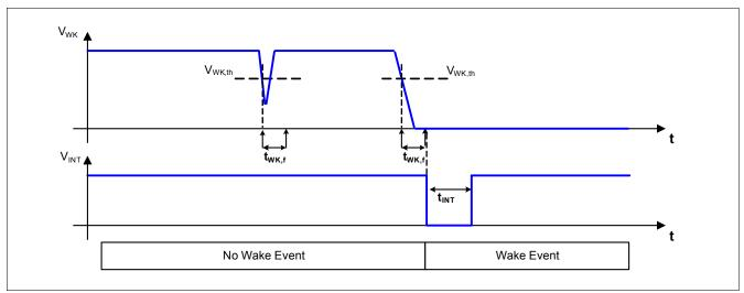
Figure 31 shows a typical wake-up timing and filtering of transient pulses.
