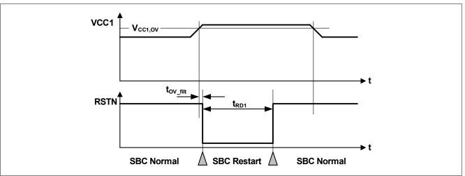
Figure 43 VCC1 Over Voltage Timing Diagram
