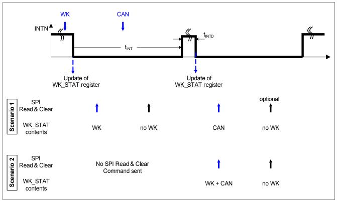
Figure 34 Interrupt Signalization Behavior
