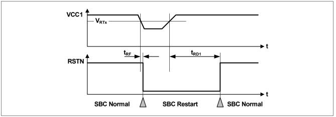
Figure 42 VCC1 Undervoltage Timing Diagram
