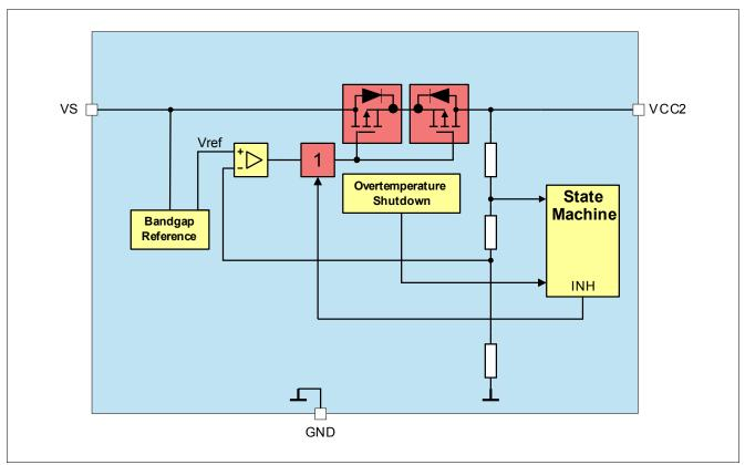
Figure 20 Module Block Diagram
