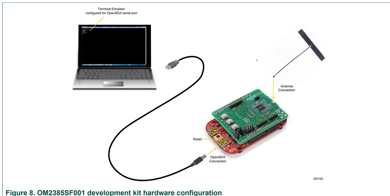
Figure 8. OM2385SF001 development kit hardware configuration
