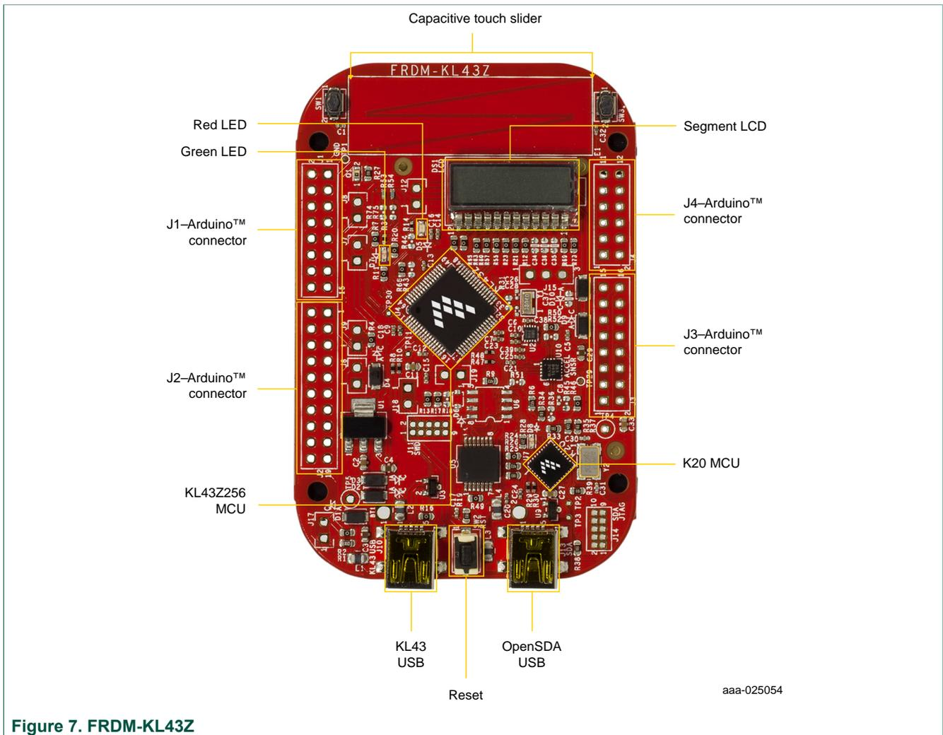
A single row of Arduino™ connectors on the OM2385/SF001 connects to the outer row (even numbers) of the Arduino™ connectors on the FRDM-KL43Z. Table 7 describes the connections between the two boards.
