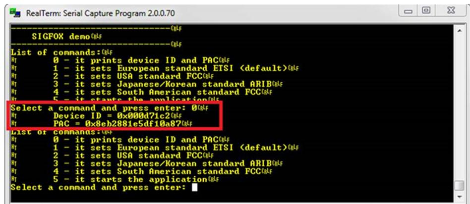
3. In the **List of commands**, select the appropriate region (**1, 2, 3** or **4**), then press **Enter**. This configures the device according to the selected regional standards. (This selection will have to be made every time the board is re-connected through the **SDA** port.)
