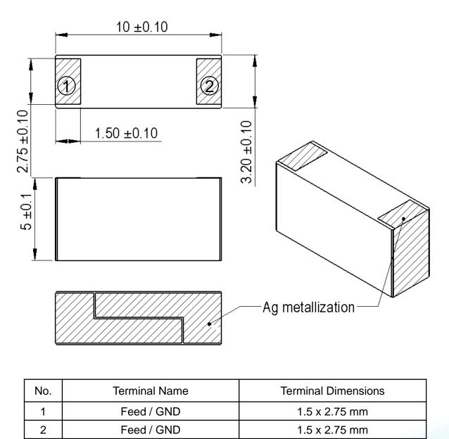
Antenna is symmetrical. Either of terminals 1 or 2 can be Feed / GND
