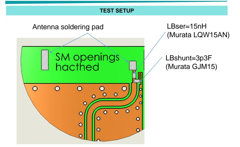
Recommended test board PCB layout for electrical characteristic measurement. Substrate material FR4, thickness 1mm
