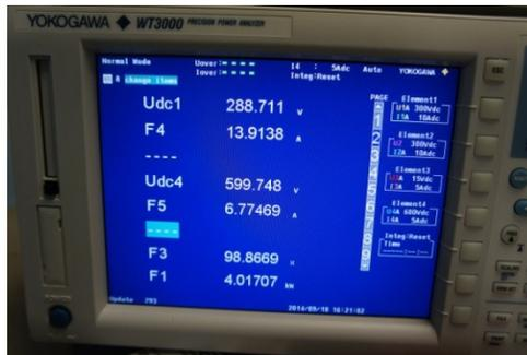
Figure 11. Efficiency data for this EVL board
