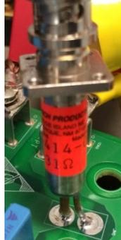
Figure 7. Low side current measurement
