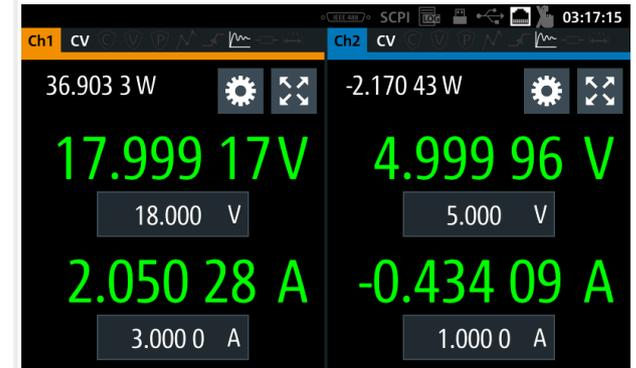
The linear design of the output stages reduces residual ripple and noise to a minimum and makes it perfect to support the development of power amplifiers and MMICs.
