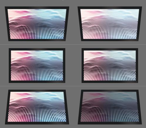
IPS technology was developed during the late 1980s to specifically address the issues with the existing TN LCDs, enabling the introduction of displays that offered increased quality colour reproduction and more accurate and consistent viewing from a wider range of angles.
