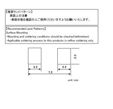
The data is reference only. Electrical characteristics vary depending on environment or measurement condition. TAIYO YUDEN reserves the right to make change to the data at any time without notice. Before making final selection, please check product specification. 2019.01.24
