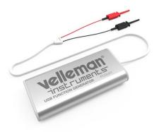
The PC USB miniature function generator is simple to use and has a frequency range of up to 1 MHz!
