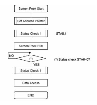
Note: This command is available when hardware column number and software column number are the same. Hardware column number is related to MD2 and MD3 setting. Software column number is related to Set Text Area and Set Graphic Area command.
