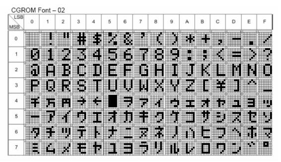
The RA6963 has two part number - RA6963L2NA and RA6963L2NB. The RA6963L2NA is compatible to T6963C(code 0101) and the default font is Figure 6-13 as above. The RA6963L2NB is compatible to T6963C(code 0201) and the default font is Figure 6-14 as above.
