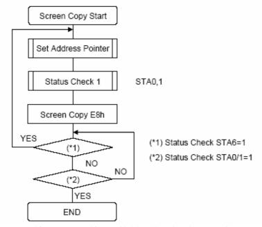
Note: This command is available when hardware column number is the same. Hardware column number is related to MD2 and MD3 setting. Software column number is related to Set Text Area and Set Graphic Area command.
