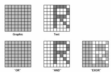
Note: Attribute functions can only be applied to text display, since the attribute data is placed in the graphic RAM area.
