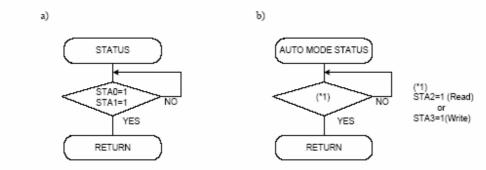
Note 4: When using the MSB=0 command, a Status Read must be performed.
