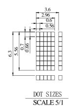
The non-specified tolerance of dimension is  $\pm 0.3 \text{ mm}$ .
