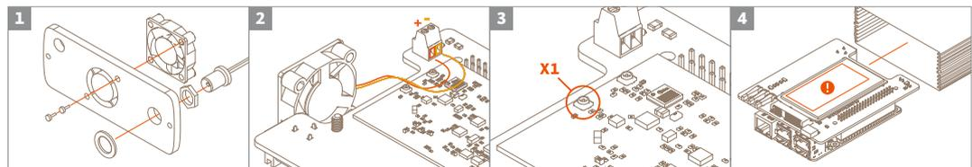
1. Insert the SD card then attach the fan as shown in the picture then screw together the enclosure panel with the SMA pigtail.
