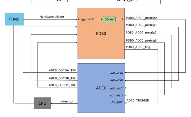
Figure 2. Inter-connectivity diagram in back-to-back mode
