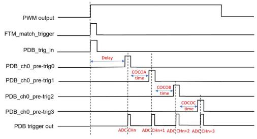
Figure 3. Timing of PDB trigger and pre-trigger outputs to ADC
