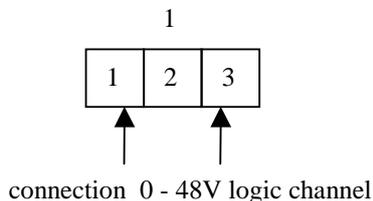
by a screw terminal between the points 1 and 3 of the screw terminal box
