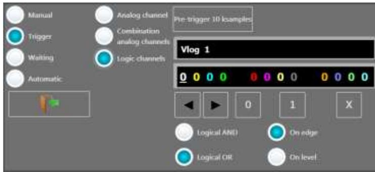
The 12 logic channels can be used in the trigger word:
