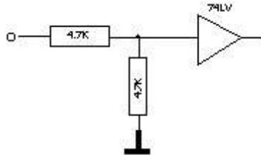
Non-connected inputs are 0V potential (level 0).
