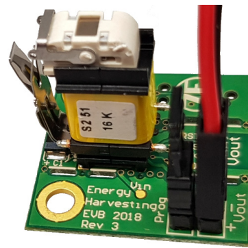
Figure 6. Power Connection and Programming Mode Jumper
