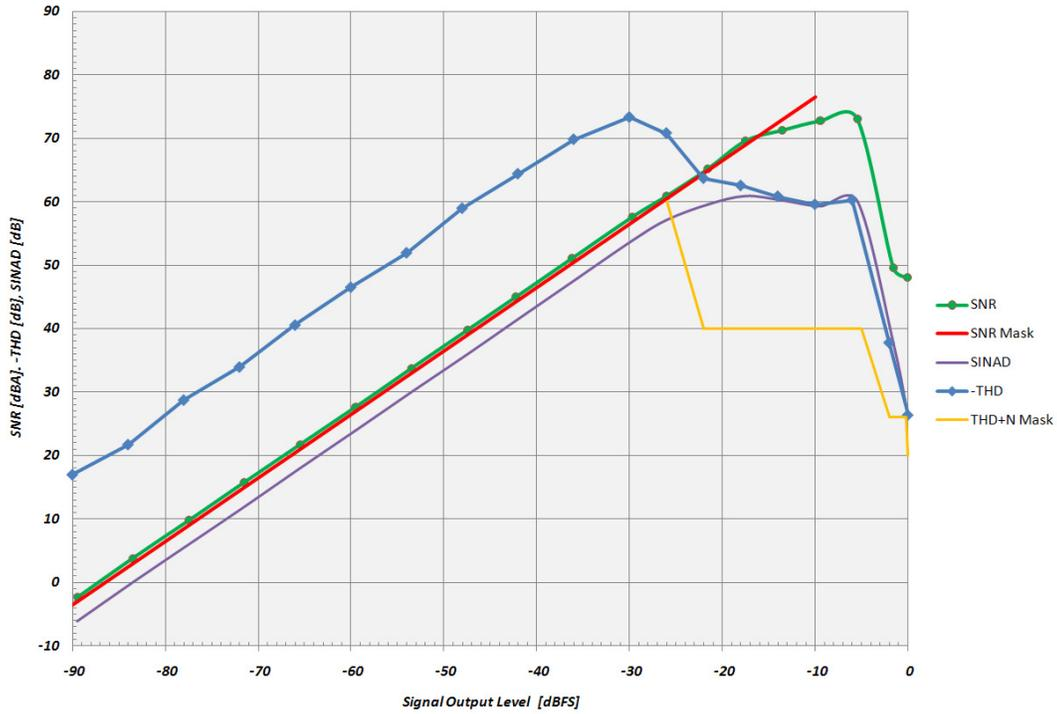
Figure 5. THD, SINAD and SNR vs. Output Level
