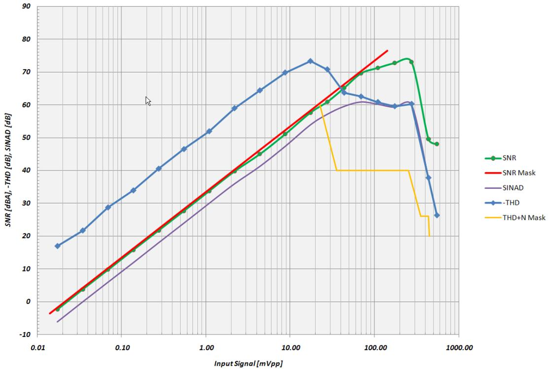
Figure 4. THD, SINDA, and SNR vs. Input Amplitude
