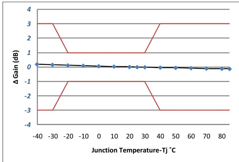
Figure 6. Δ Gain vs. Temperature (Nominal Temperature = 25°C)
