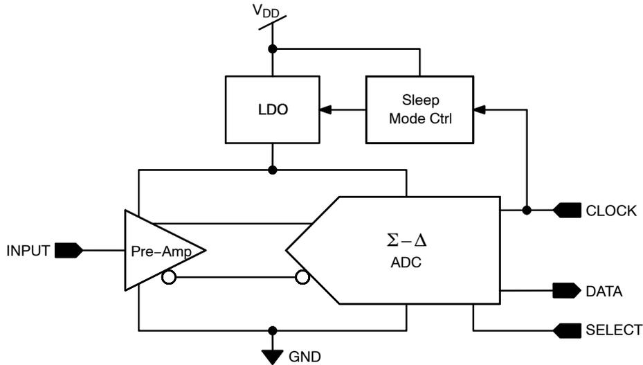
Figure 1. Block Diagram
