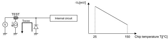
Figure 7. Model diagram for measuring chip temperature
