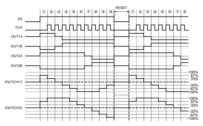
CW\_CCW Switch Timing Chart (FULL STEP, MODE0=L, MODE1=L, ENABLE=H)
