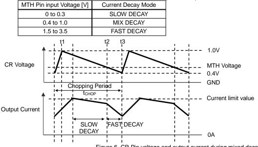
Figure 6. CR Pin voltage and output current during mixed decay
