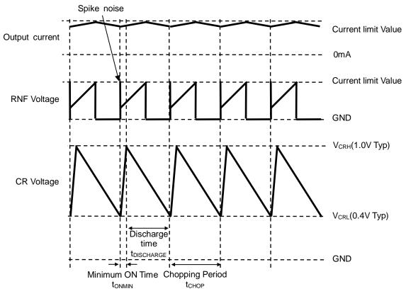
Figure 4. Timing chart of CR voltage, RNF voltage and output current
