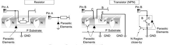
Figure 10. Example of monolithic IC structure
