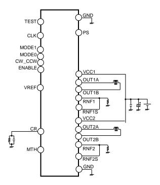
Figure 1. BD60223FP application circuit diagram
