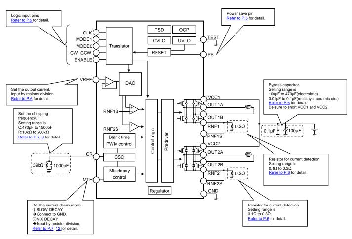
Figure 8. BD60223FP block diagram and applied circuit diagram
