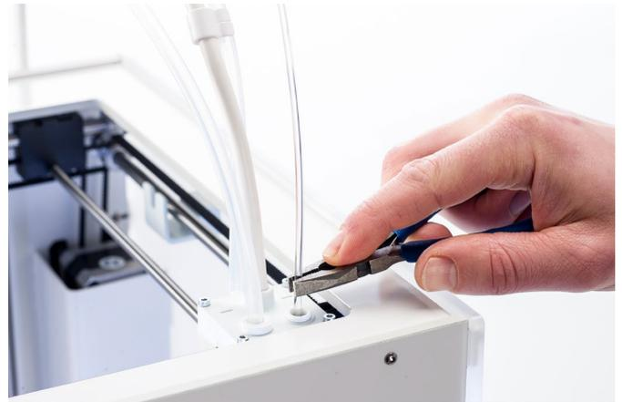
4. Cut off the tip of the filament that you have just pulled out.
