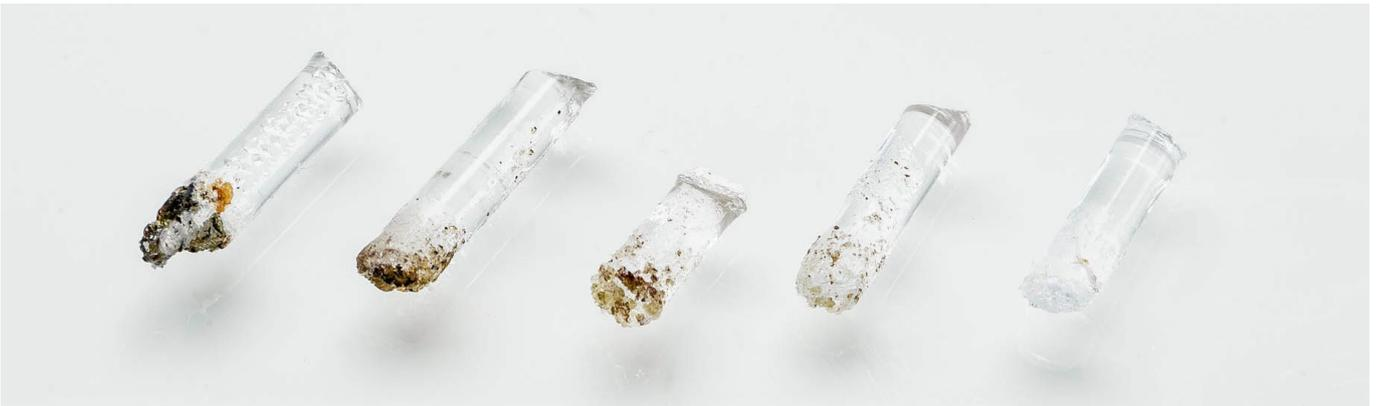
6. Repeat this procedure until there is no more degraded material visible on the tip of the cleaning filament. The tip of the filament should look as clean as the example on the right.
