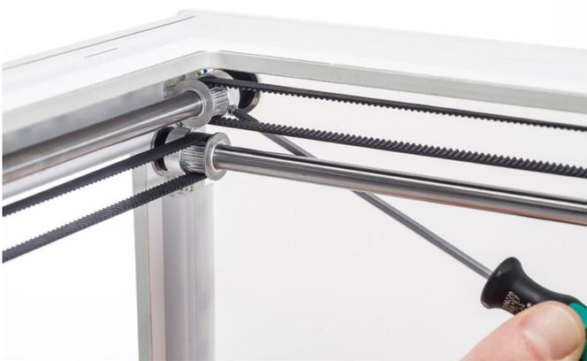
The axles should not move at all. If one of the axles does move, you can observe a ticking noise of the pulleys hitting the frame. In this case it is recommended to calibrate the print head. For instructions on how to do this, take a look at the [Ultimaker website](#).
