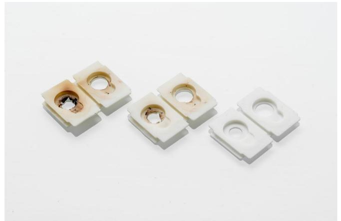
According to these images, it is highly recommended to replace the cover on the left and advisable to replace the cover in the middle. The cover on the right is in perfect condition and will not need to be replaced. Instructions on how to replace the silicone nozzle cover can be found on the [Ultimaker website](#).
