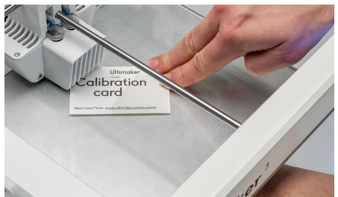
After calibrating the build plate with the first nozzle, the second nozzle needs to be aligned as well, to ensure the heights of both nozzles are set correctly. For this it is only necessary to set the correct height by using the calibration card.
