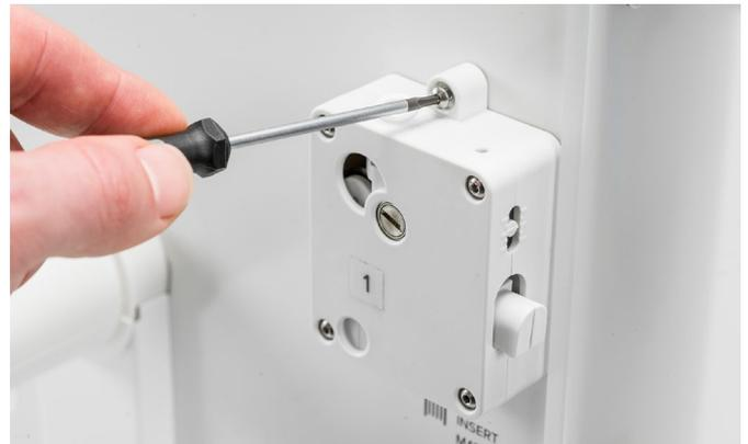
5. Open the feeder by removing the four bolts that hold the housing parts together. Place the two halves in front of you, making sure that all parts are in the back section of the feeder.
