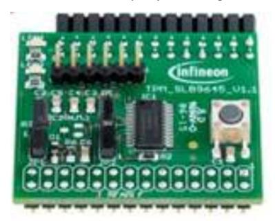
Infineon's Trusted Platform Module (TPM) SLB 9645 is a fully TCG standard compliant TPM 1.2.
